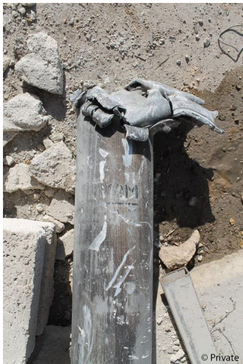
Remnant of a rocket that hit the al-Masaken neighbourhood on 16 June 2015. According to weapons experts, it is part of a 122mm Grad rocket.
